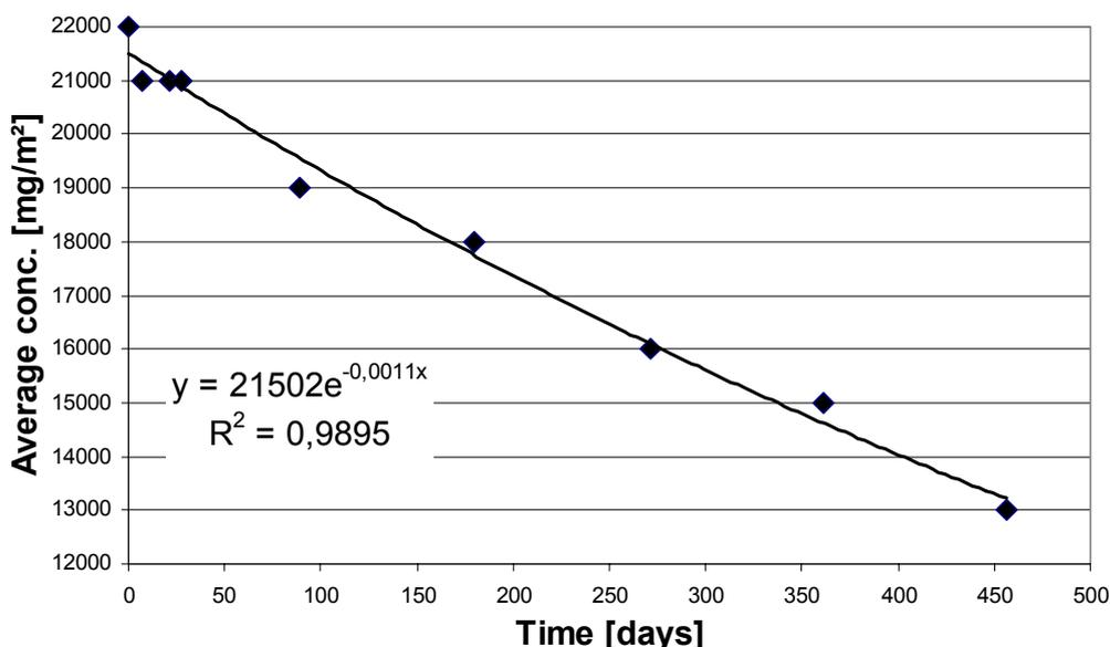
**Figure 1.** Decay curve for chlorpyrifos, sprayed onto glass plates (Average conc.= 3 samples)
